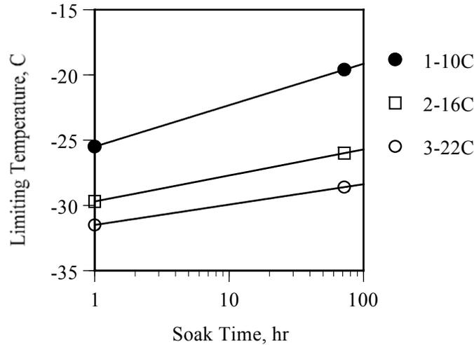
**Figure 6. Physical Ageing Rates for Binders Used on C-SHRP Test Sections on Highway 631**
