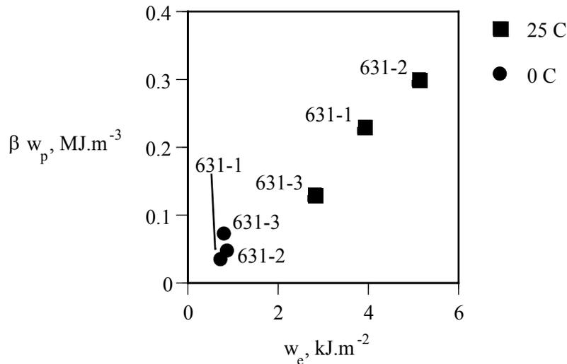
**Figure 9. Fracture Energies in Ductile State for Recovered Binders from Highway 631**
