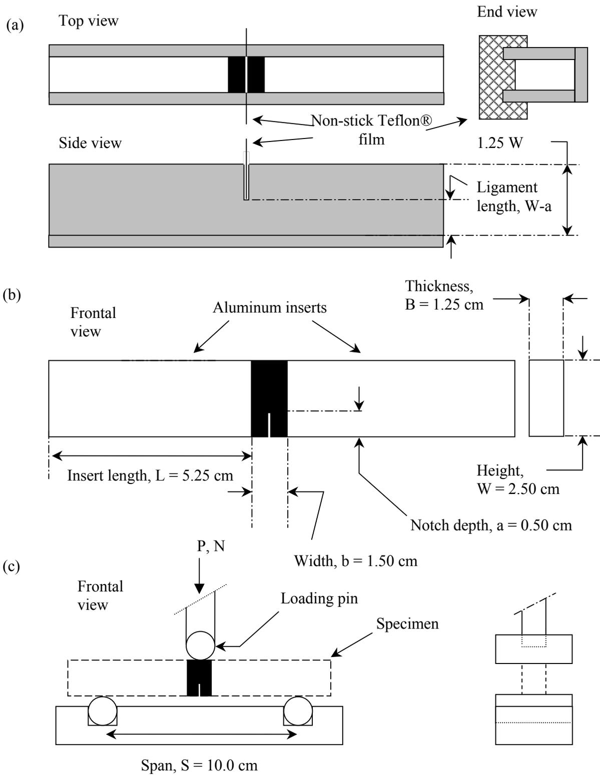
**Figure 4. Fracture Test for Asphalt Binders: (a) Mold Design; (b) Sample Dimensions; and (c) Three-Point Bend Test Setup**
