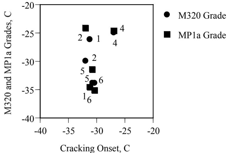
**Figure 1. Comparison Between AASHTO M320 and MP1a Grade Temperatures and Cracking Onset Temperatures as Measured at 12-mm Depth**
