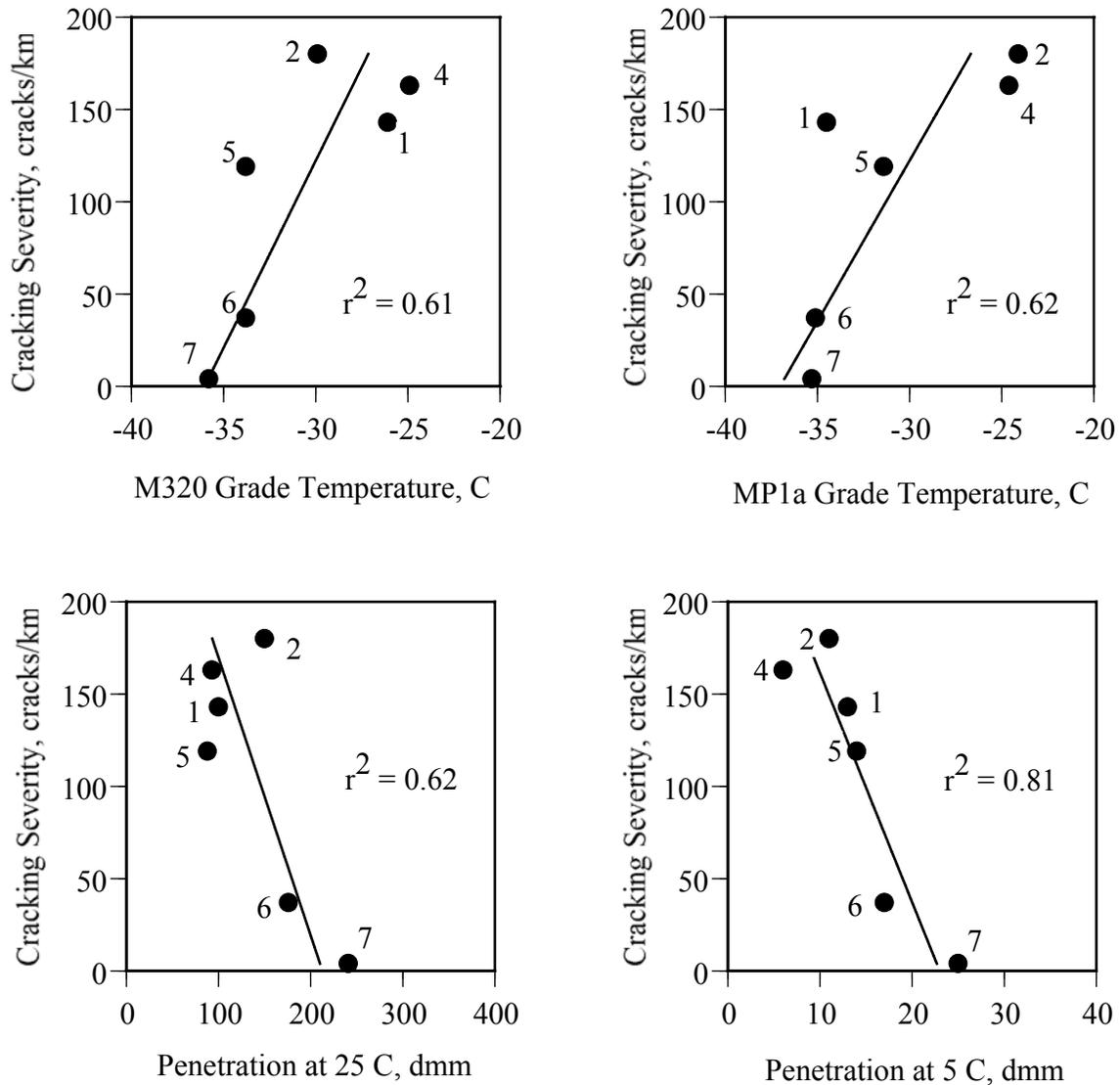
**Figure 2. Correlations Between Cracking Severity and AASHTO M320, MP1a and Penetration Values at 25°C and 5°C for Lamont, Alberta Test Sections**
