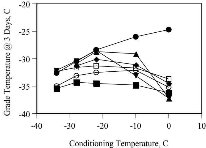
**Figure 15. Continuous Grade Temperatures after 3 Days Conditioning for Highway 655 Binders**
