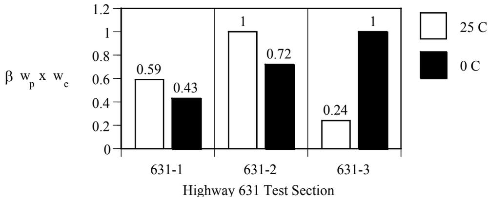
**Figure 10. Relative Ductile Fracture Performance of C-SHRP Binders from Highway 631**
