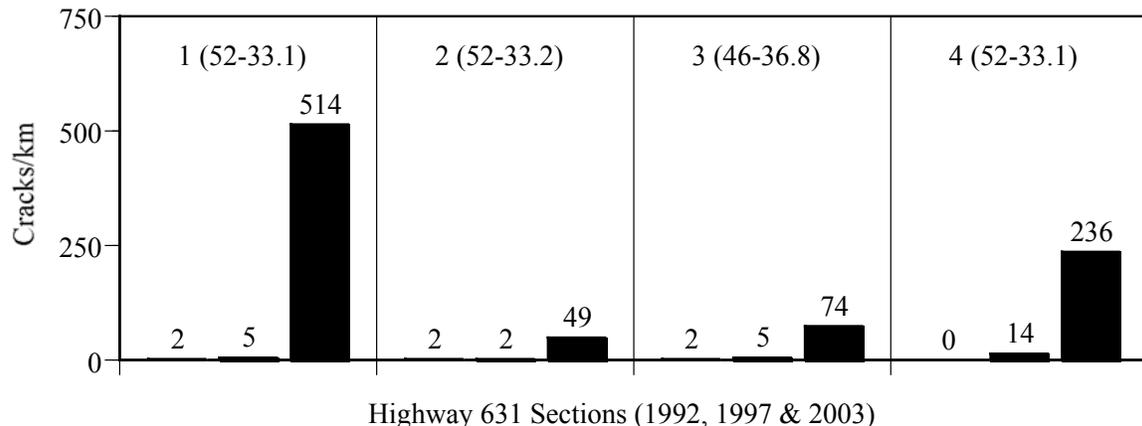
**Figure 3. Cracking History for the C-SHRP Test Road on Highway 631 near Hearst, Ontario**
