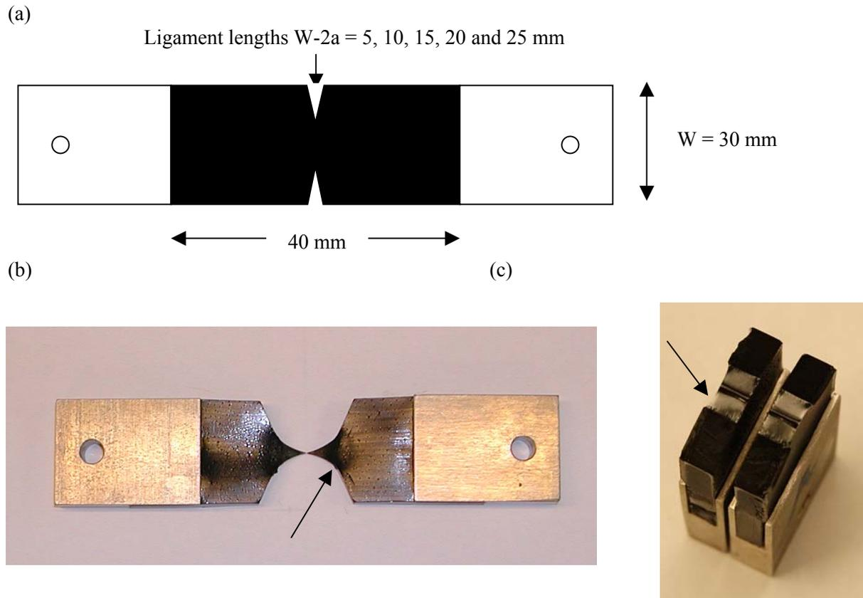
**Figure 5. (a) Schematic of Double-Edge-Notched Tension (DENT) Specimen Design, (b) Photograph of Sample after Ductile Failure, and (c) Photograph of Sample after Failure at  $0^\circ\text{C}$**
