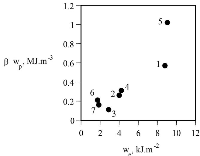
**Figure 16. Fracture Energies in Ductile State for PAV-aged Highway 655 Binders**
