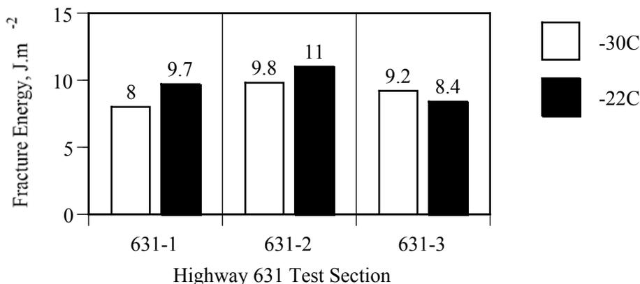
**Figure 8. Fracture Energies in Brittle State for Recovered Binders from Highway 631**
